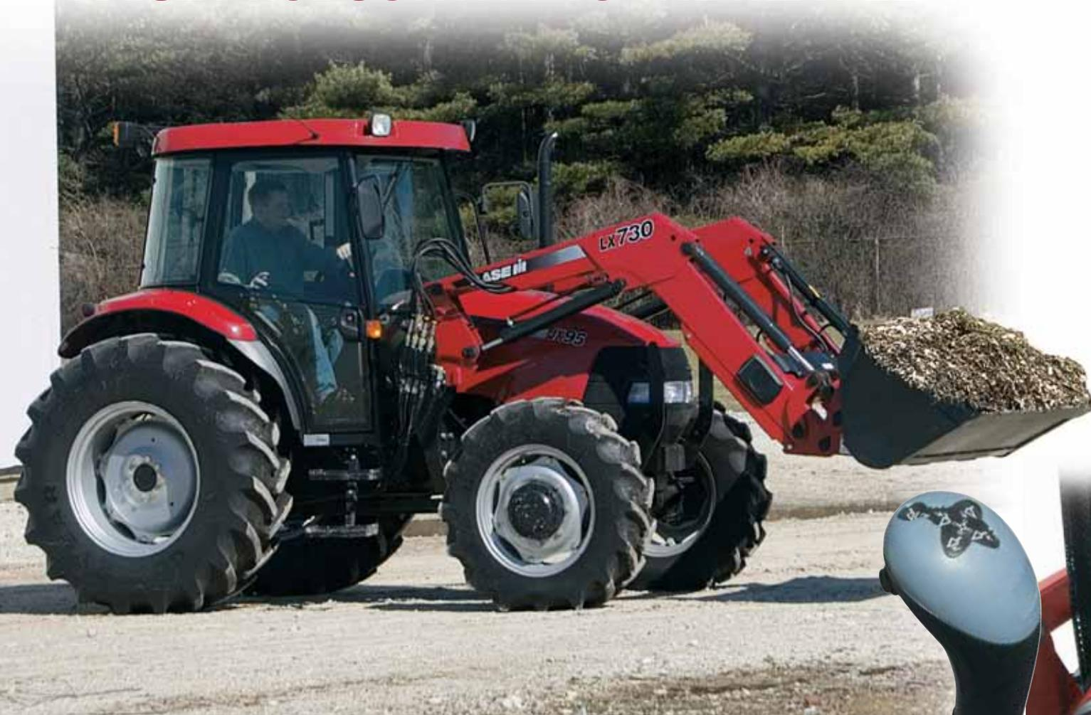
Nothing speeds up cycle times faster than this **4-way joystick control** for loader operation. Keep it in your right hand and let your left hand shuttle from forward to reverse and back again. A button on the joystick lets you control a third device such as a grapple or bale hugger.
