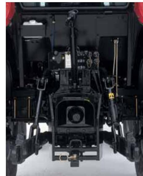
▲ **Plug in to the dedicated hydraulic system** to get 13.6 gpm (51.7 L/min) at the rear. One remote is standard; two or three are optional.
