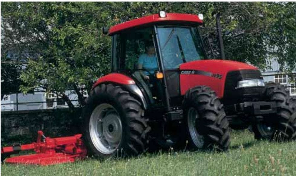
JX Series tractors from Case IH are built to get the job done in any application — mowing, baling, box blading, or loader chores. With dedicated hydraulics, heavy-duty 3-point hitch and powerful PTO, these tractors can tackle just about any task you find around the farm, field or feedlot.
