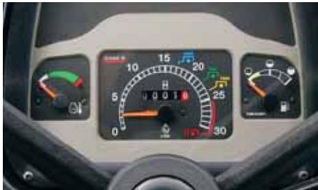
▲ **An analog instrument cluster** includes the following warning lights: water in fuel, engine oil pressure, alternator, PTO engaged, turn indicators, headlamp main beam, restricted air cleaner, parking brake, and tail lights indicator.
