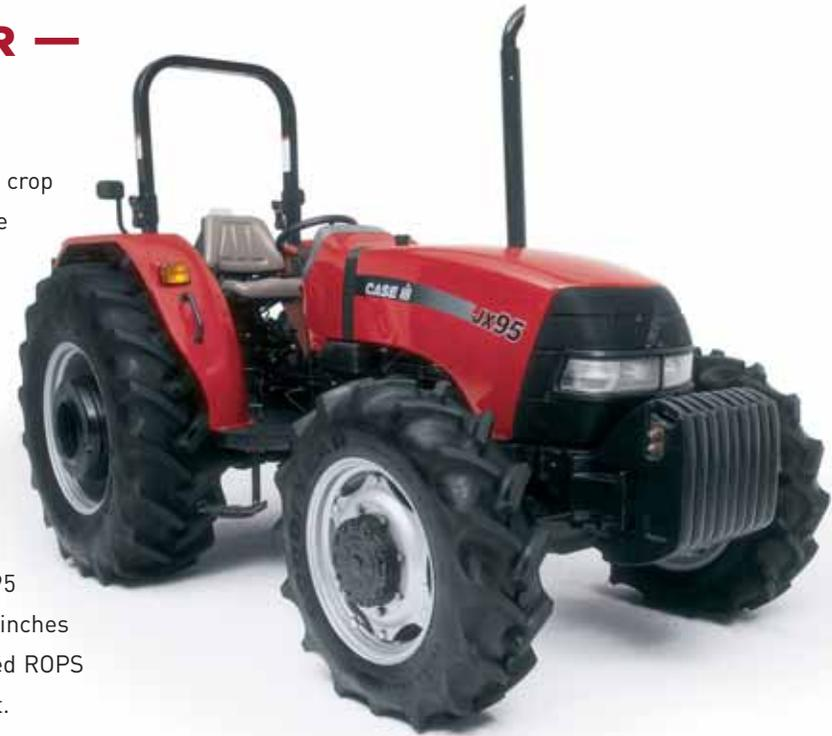
▲ **Straddle deck** offers lower overall clearance than flat deck models. A dedicated left-hand shuttle and 12x12 transmission are both standard features.
