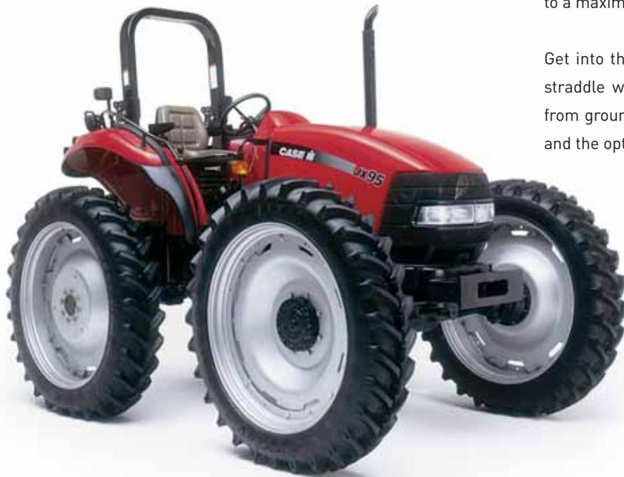
▲ **High Clear** offers optional axle spacers to provide up to 99 inch row spacing.
