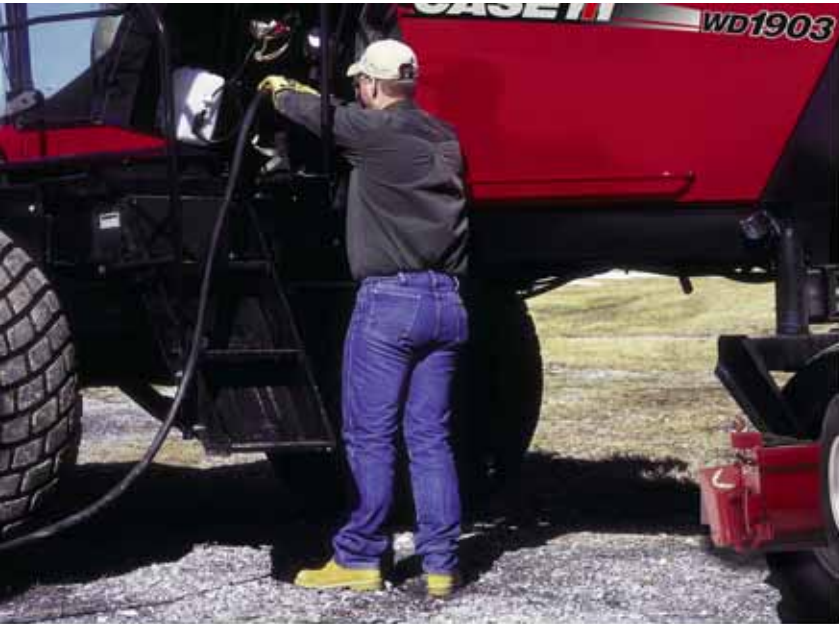
With a fuel capacity of 120 gallons (454 liters), you'll be on the move all day long without refills. The fuel fill and hydraulic reservoir can be reached easily from the ground.
