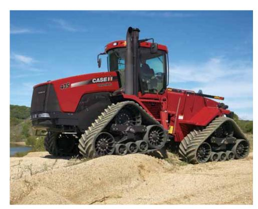
▲ The QUADTRAC tractor **oscillates up to 26 degrees** to walkover uneven terrain while keeping tractor weight evenly distributed for more traction. Tracks **pivot up to 20 degrees** vertically to ensure soil contact, greater flotation, less compaction, superior traction and an industry-leading ride. And QUADTRAC easily walks over uneven terrain without a "break-over" point typical of competitive two-track systems.
