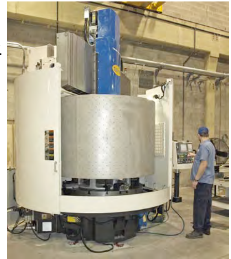
large 72" ringless duplex SS basket on VTL
