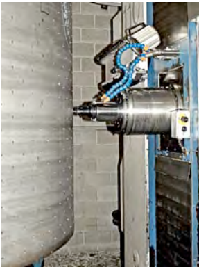
drilling thousands of holes into the side sheet
