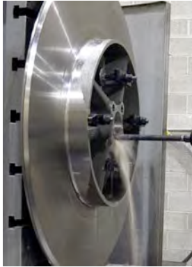
drilling a basket hub
