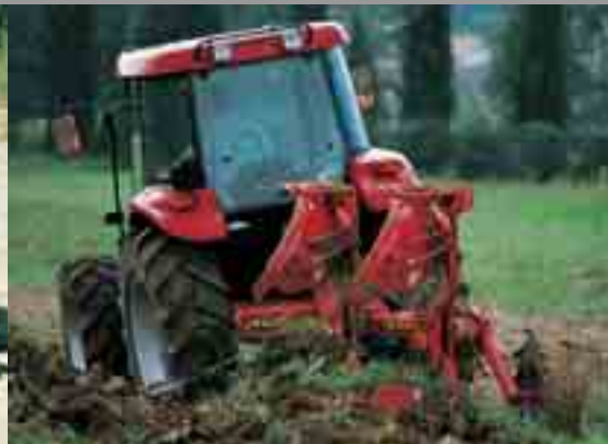
Maximum tractive effort is achieved due to four-wheel drive and differential locks.
