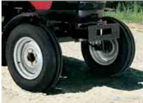
An adjustable two-wheel drive axle with 8 track settings is available.
